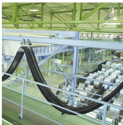
Energy and data transmission on a steel-mill-crane
