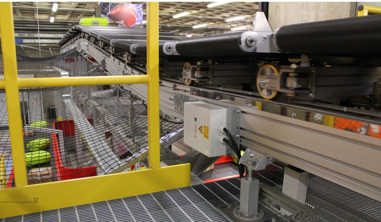
**Cross-belt or tilt-tray sorters** both in baggage handling systems and parcel sortation have to be extremely reliable and are designed for constant, high-speed operation of up to 3 m/s.
