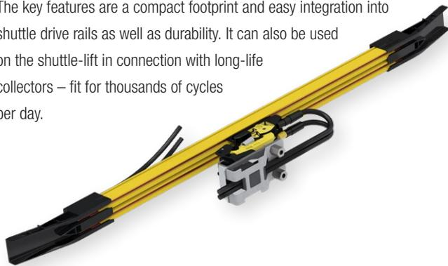
**MultiLine 0831** is a compact conductor rail used for pallet shuttles carrying higher loads and operating with alternating current. It features a compact 3-, 4- or 5-pole insulation with pre-mounted connectors for fast assembly.
